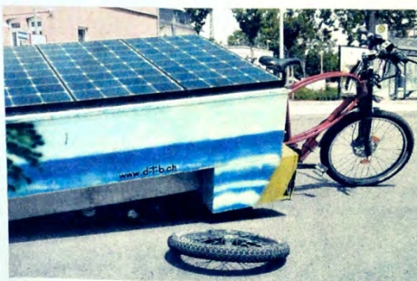
The solar trike had two broken axles after 500 km – the right axle went in the middle of a busy street in Osthofen – but luckily causing no accident or injury!
